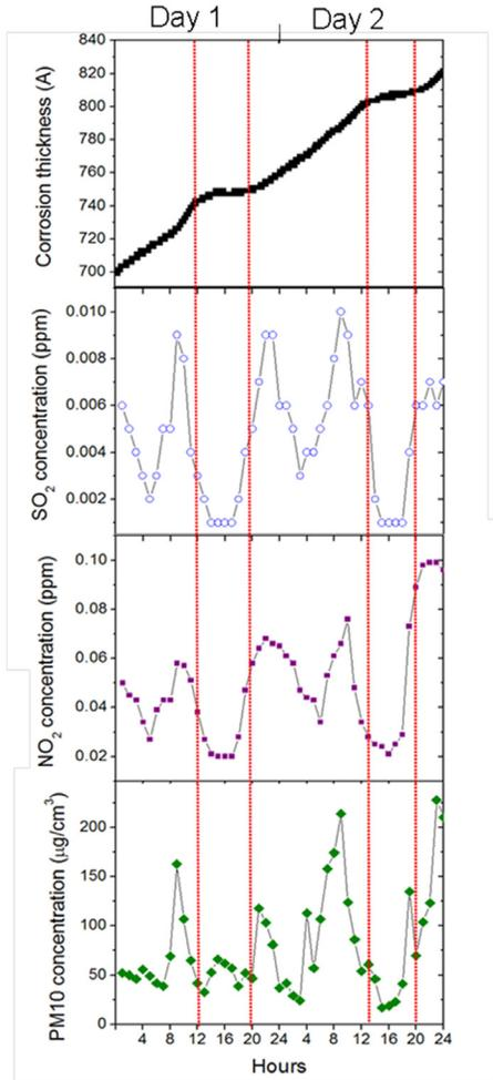
**Figure 5** Silver corrosion thickness, SO<sub>2</sub>, NO<sub>2</sub>, and dust level as a function of time of day in a data center.
