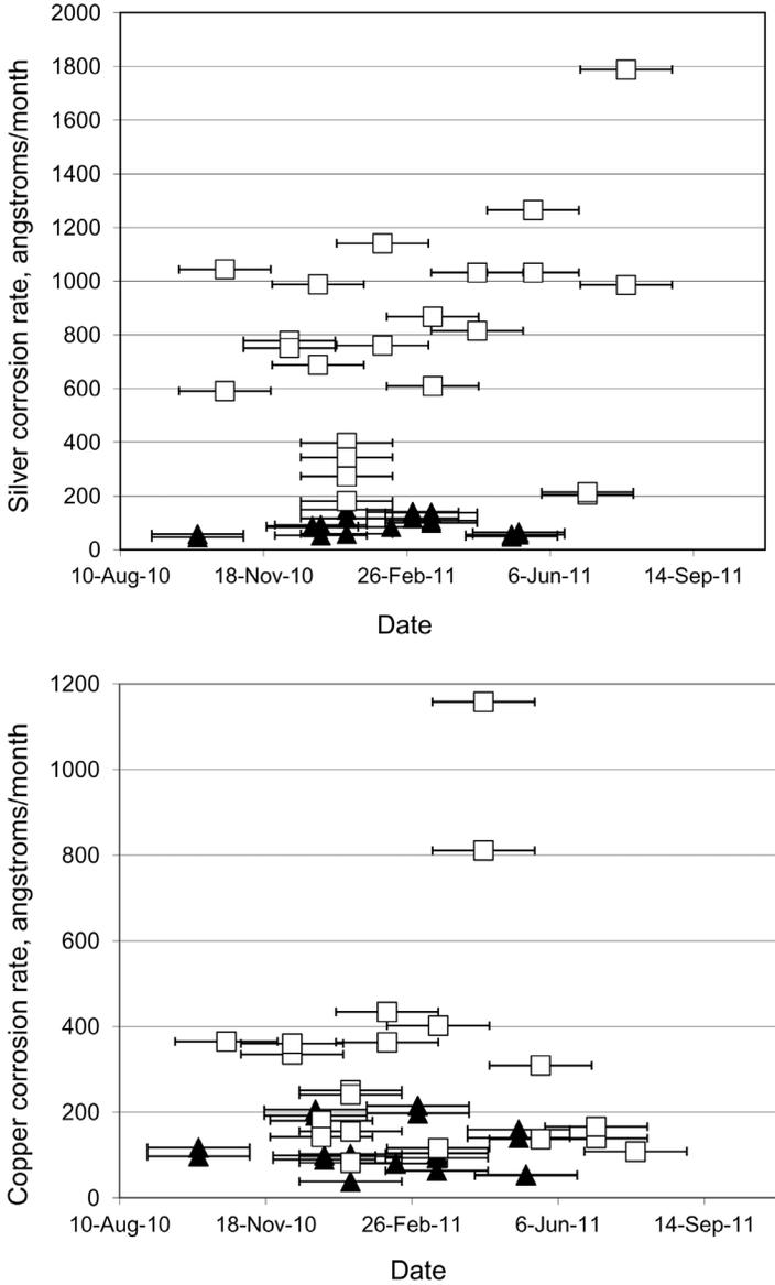
**Figure 4** The open square data points are for data centers with known corrosion-related hardware failures. The solid triangle data points are for data centers with no known corrosion-related hardware failures. Notice that the silver corrosion rates for data centers with and without corrosion-related hardware failures show no overlap; whereas, the copper corrosion rates for the two types of data centers show some overlap.
