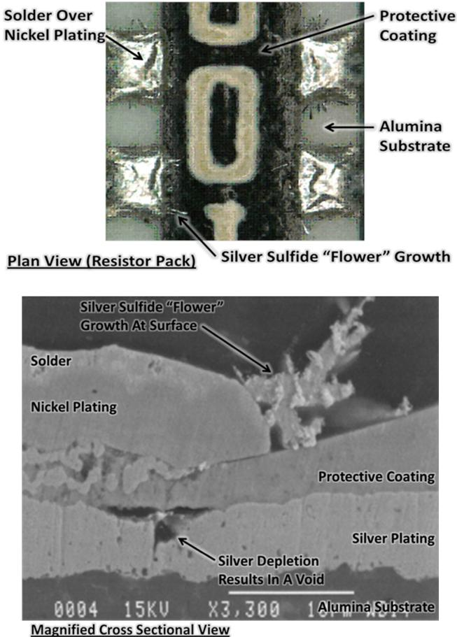
**Figure 2** (Top) plan view and (bottom) magnified cross-sectional view of an example of a component failure due to an environment high in sulfur-bearing gases attacking the silver metallization in the component, producing silver sulfide “flowers.”
